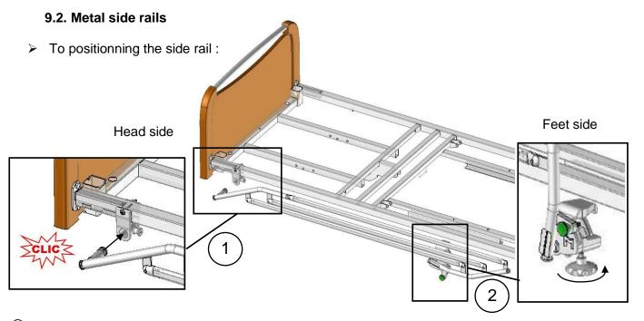
①Insert amount of the side rail folded in the grip jaw on the head side of the bed to hear "CLIC".
