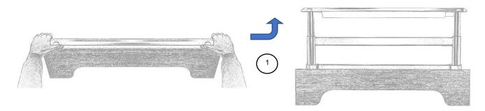
② Check that the side rail is locked by trying to fold it without using the unlocking buttons.
