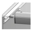
Unique telescopic cart to compensate for varrying wall widths.
